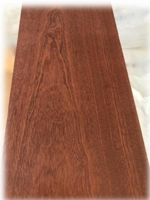
Illustration 1; Mahogany veneer coated in matt with the above system (primer, sealer, basecoat and protective varnish)
