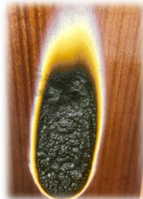
Illustration 2; Intumescent protective layer after exposure to fire.
